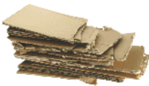
Corrugated Cardboard (Wavy center layer)
