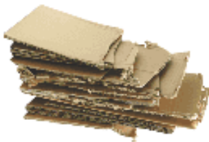
Corrugated Cardboard (Wavy center layer)
